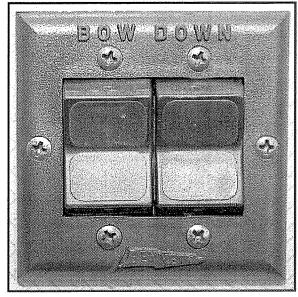
Once the best bow cruising attitude is achieved, activate the port or starboard trim switches individually to correct for unequal lateral loading. Do not use trim tabs to compensate for excessive unequal weight distribution.
