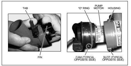
3. Check the reinstallation by trying to twist the fins counter-clockwise *without* lifting the tab; the pump motor should stay in place.
