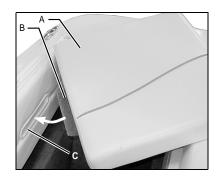
**Step - 3:** Press down firmly on the inboard side of each jump seat until they rest firmly on the motorbox ledges.
