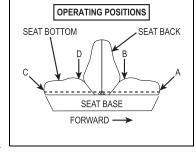
6. Lock the aft seat into position by pushing down at point (C).
