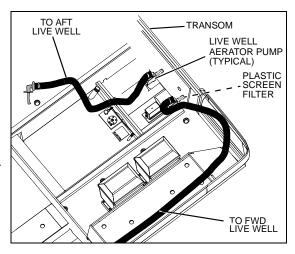
ing adequate amounts of water. If there appears to be a problem, check the system, including the plastic screens over the transom intakes for weeds or other debris.
