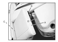
**Step - 3:** Press down firmly on each jump seat until they rest firmly on the cockpit and motor box ledges.
