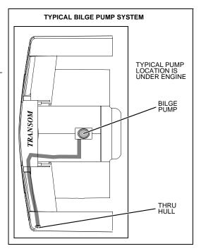
If the bilge pump hose is not the problem, check the bilge pump housing for clogging debris:
