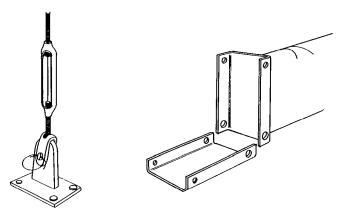
8. Bolt the mast to the mast tabernacle. Raise the mast and attach the forestay and the lower shrouds.
