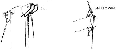
4. Attach the backstay, forestay, upper and lower shrouds to the mast. Safety wire the upper shrouds in the slots at the end of the spreaders. The shrouds should be able to run freely in the slots but they should be wired so they will not come out of the slots. 5. Loosen the turnbuckles until four threads are showing in each end of the turnbuckle barrel.
