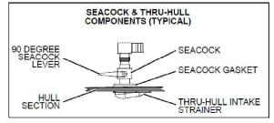
Before using any system with a seacock, make sure the seacock is Open and stays Open until the system is shut Off.
