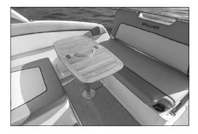
When not in use, store the table and table leg under the aft seat cushion. Secure the table in place with the provided cord.
