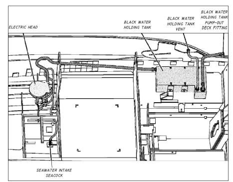
• Keep the intake seacock *Closed* while your boat is underway or when the system will not be used for long periods of time.
