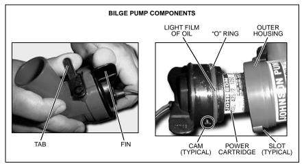
3. Check the reinstallation by trying to twist the fins counter-clockwise without lifting the tab; the cartridge should stay in place.
