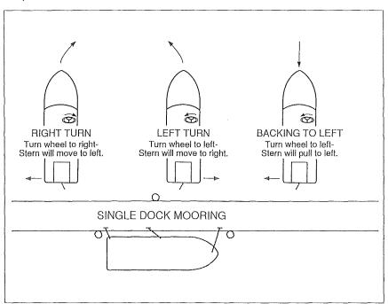
Proper docking requires preparation. Start by making sure you have adequate mooring gear, and that it is stowed correctly and ready for use. Your dealer is the best source for information concerning the amount and type of equipment you should carry.
